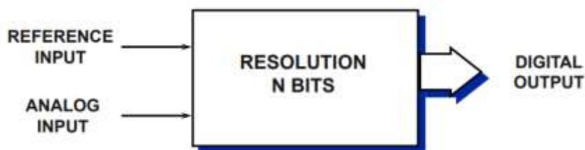
$$\text{DIGITAL OUTPUT CODE} = \frac{\text{Analog Input}}{\text{Reference Input}} \times (2^N - 1)$$
