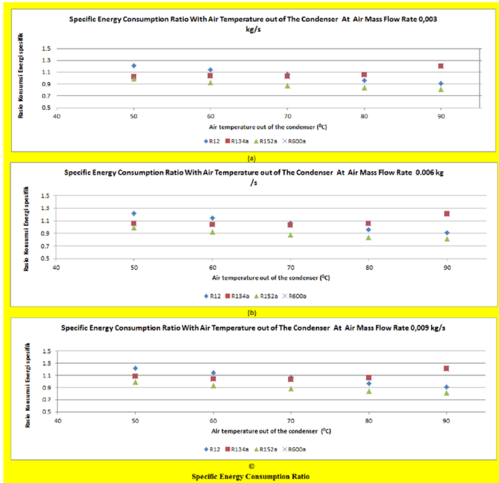
FIGURE 2. Graph of Energy Specific Consumptions and Ratio of Energy Specific Consumptions from R-134a, R-12, R-152a and R-600a Refrigerants
