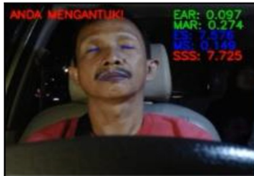
Figure 3.20: Sleepines driver noticed from image processing SLIFA device
