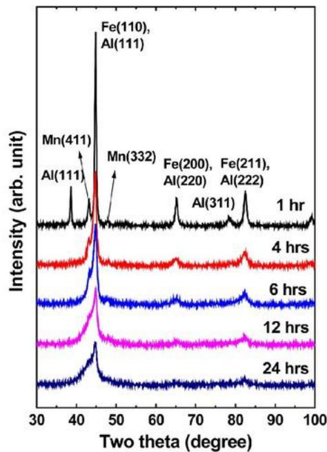
Fig. 1. XRD profiles of mechanically alloyed  $\text{Fe}_{55}\text{Al}_{35}\text{Mn}_{10}$  powder with milling time.
