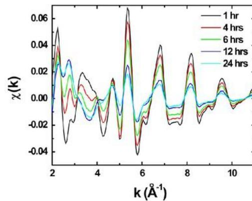
Fig. 2. EXAFS spectra of  $\text{Fe}_{55}\text{Al}_{35}\text{Mn}_{10}$  alloys with milling time.
