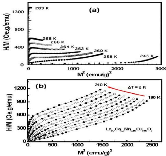
**Figure 5.**  $H/M$  versus  $M^2$  plots of the isotherms for (a)  $\text{La}_{0.7}\text{Ca}_{0.3}\text{MnO}_3$  (after Mira *et al.* [4]), and (b)  $\text{La}_{0.7}\text{Ca}_{0.3}\text{Mn}_{0.95}\text{Cu}_{0.05}\text{O}_3$ . While the negative slope can be found in (a)  $\text{La}_{0.7}\text{Ca}_{0.3}\text{MnO}_3$  at some temperatures, only the positive slope is found in (b)  $\text{La}_{0.7}\text{Ca}_{0.3}\text{Mn}_{0.95}\text{Cu}_{0.05}\text{O}_3$ .
