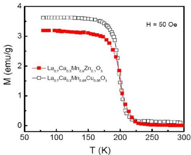
Figure 3. Temperature dependence of the zero-field cooled magnetization for  $\text{La}_{0.7}\text{Ca}_{0.3}\text{Mn}_{0.9}\text{Zn}_{0.1}\text{O}_3$  and  $\text{La}_{0.7}\text{Ca}_{0.3}\text{Mn}_{0.95}\text{Cu}_{0.05}\text{O}_3$  under an applied field of 50 Oe. 31
