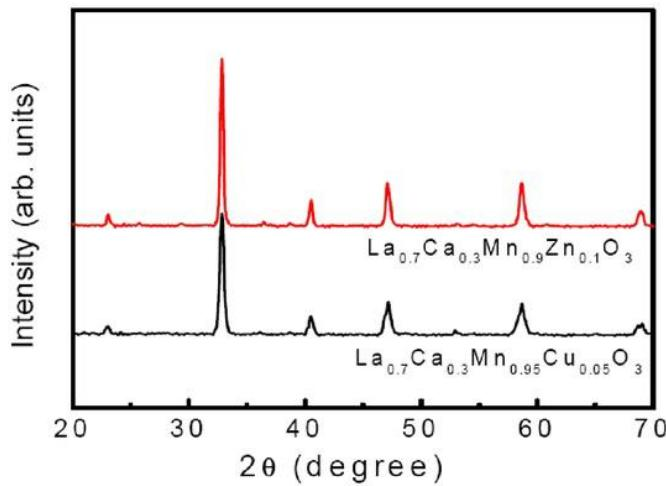
Figure 2. XRD patterns of  $\text{La}_{0.7}\text{Ca}_{0.3}\text{Mn}_{0.9}\text{Zn}_{0.1}\text{O}_3$  and  $\text{La}_{0.7}\text{Ca}_{0.3}\text{Mn}_{0.95}\text{Cu}_{0.05}\text{O}_3$ . The samples are the single phase in an orthorhombic structure (the space group  $Pnma$ ). 42
