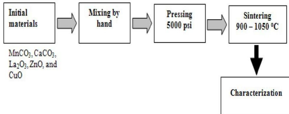
Figure 1. Diagram shows preparation of La<sub>0.7</sub>Ca<sub>0.3</sub>Mn<sub>1-x</sub>(Zn,Cu)<sub>x</sub>O<sub>3</sub> bulks.
