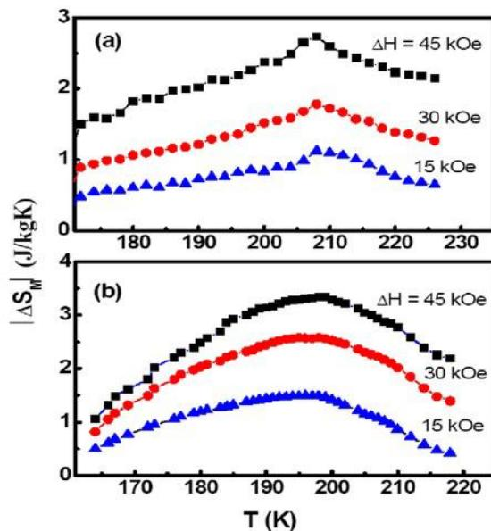
Figure 4. Temperature dependences of the magnetic-entropy change for (a)  $\text{La}_{0.7}\text{Ca}_{0.3}\text{Mn}_{0.9}\text{Zn}_{0.1}\text{O}_3$  and (b)  $\text{La}_{0.7}\text{Ca}_{0.3}\text{Mn}_{0.95}\text{Cu}_{0.05}\text{O}_3$  under various applied fields of 15, 30, and 45 kOe.
