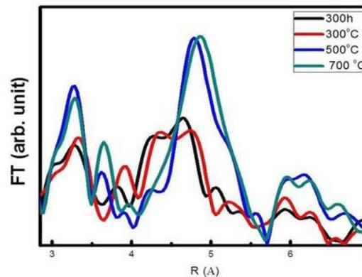
Fig. 6: The Fourier transformation of EXAFS spectra of 24 hrs milling, annealed of 300, 500, and 700°C
