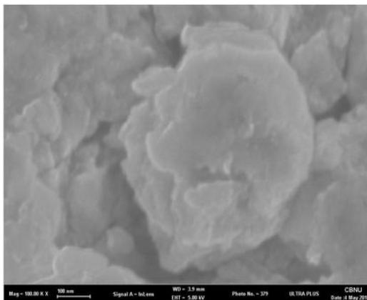
Fig. 1: Typical SEM image of nanocrystalline  $Fe_{55}Mn_{10}Al_{35}$  alloys with milling time 24 hrs
