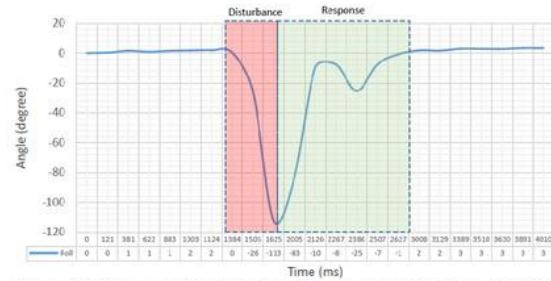
Figure 10 Response Systems for Roll Angular Position with PS-PID
