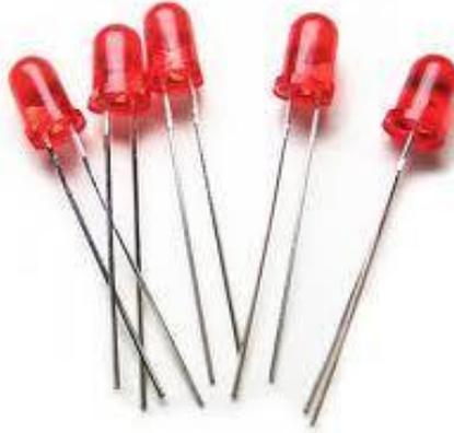
Gambar 5.2 Komponen Output Digital: LED
